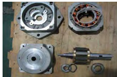
(b) Stator, rotor and other parts of built FSPM.
