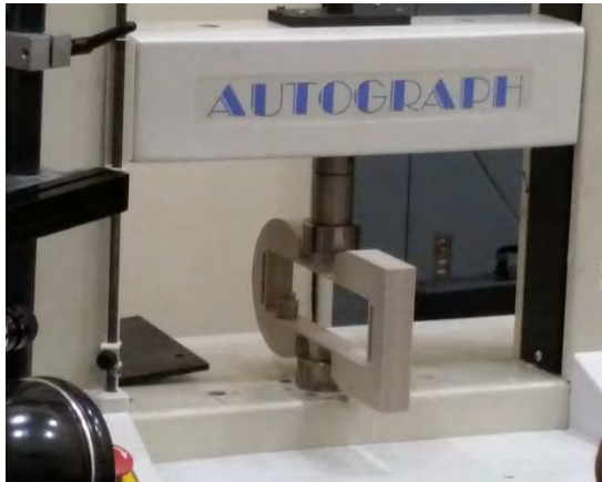
Fig. 1. Piezo-electric actuator shell compression test
