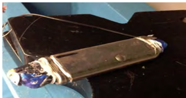
Fig. 6. A photo of a 18650 LFP battery after a crush test.
