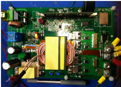
Fig. 3. Prototype of the GaN HEMT based converter.
