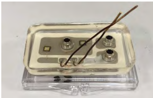
Fig. 1. Tested 10kV SiC package with thermistor and two SiC diodes
