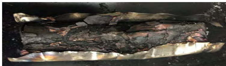
Fig. 2. A photo of the LCO 18650 battery after a nail penetration test.
