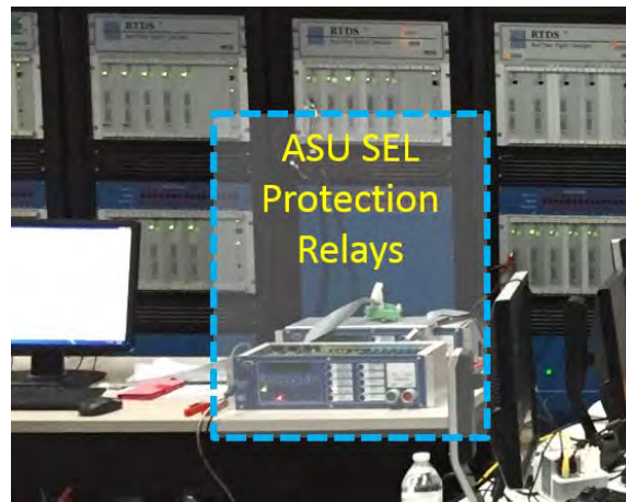
Figure 3 - ASU Protection Hardware CHIL Setup on the HIL-TB
