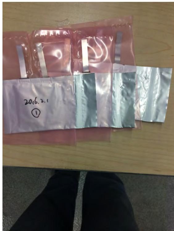
Figure 1, Photos of pouch cells of test Li-S batteries with an electrode size 23\text{cm}^2 ( 4.8\text{cm} \times 4.8\text{cm} ).
