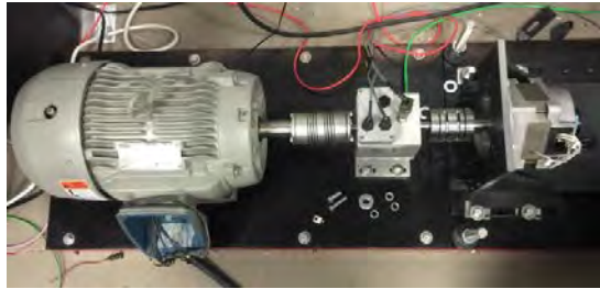
(a) Test bench with (i) dyno, (ii) torque sensor, and (iii) FSPM (from left to right).
