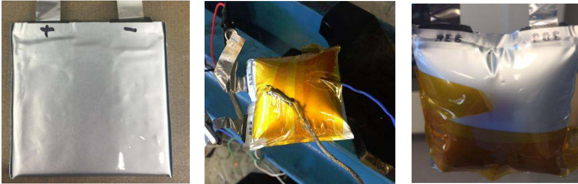
Fig. 4. LIC before (left) and after (middle and right) overcharge test
