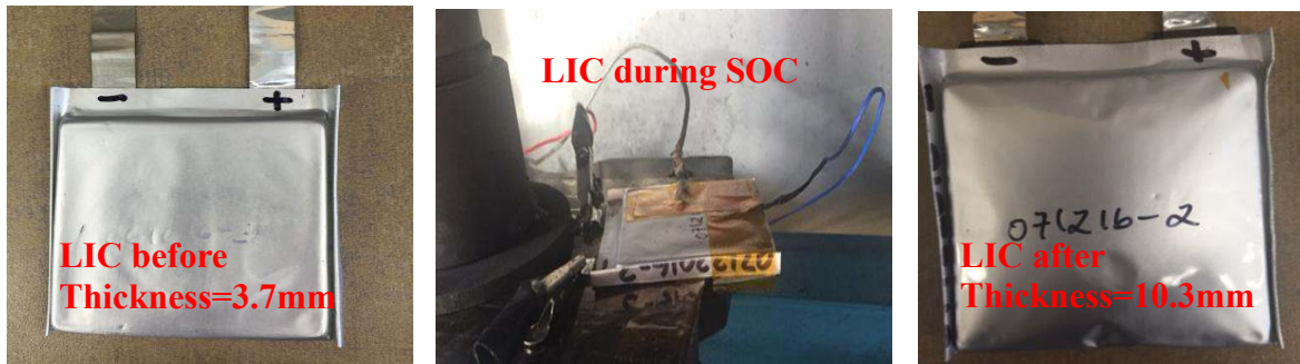
Fig. 2. LIC before (left), during (middle) and after (right) external short circuit test
