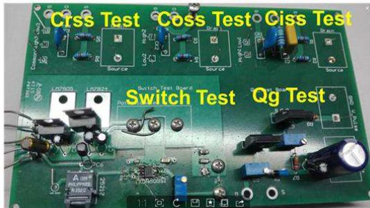
Fig. 10a: Test circuit board for the characterization of SiC MOSFET
