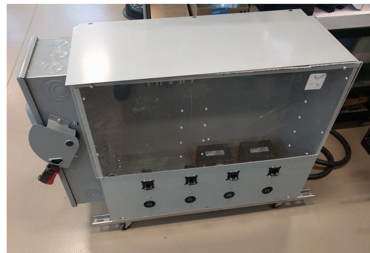
Figure 2: Grid Impedance Emulator
