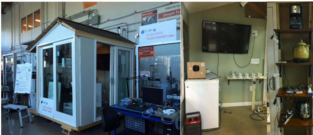
Figure 2: A residential home hardware test bed that can serve as a thermal chamber and emulate residential home load.
