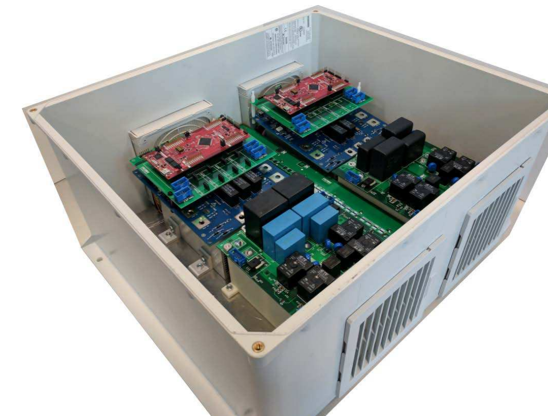
Integrated LVSSST in an enclosure
