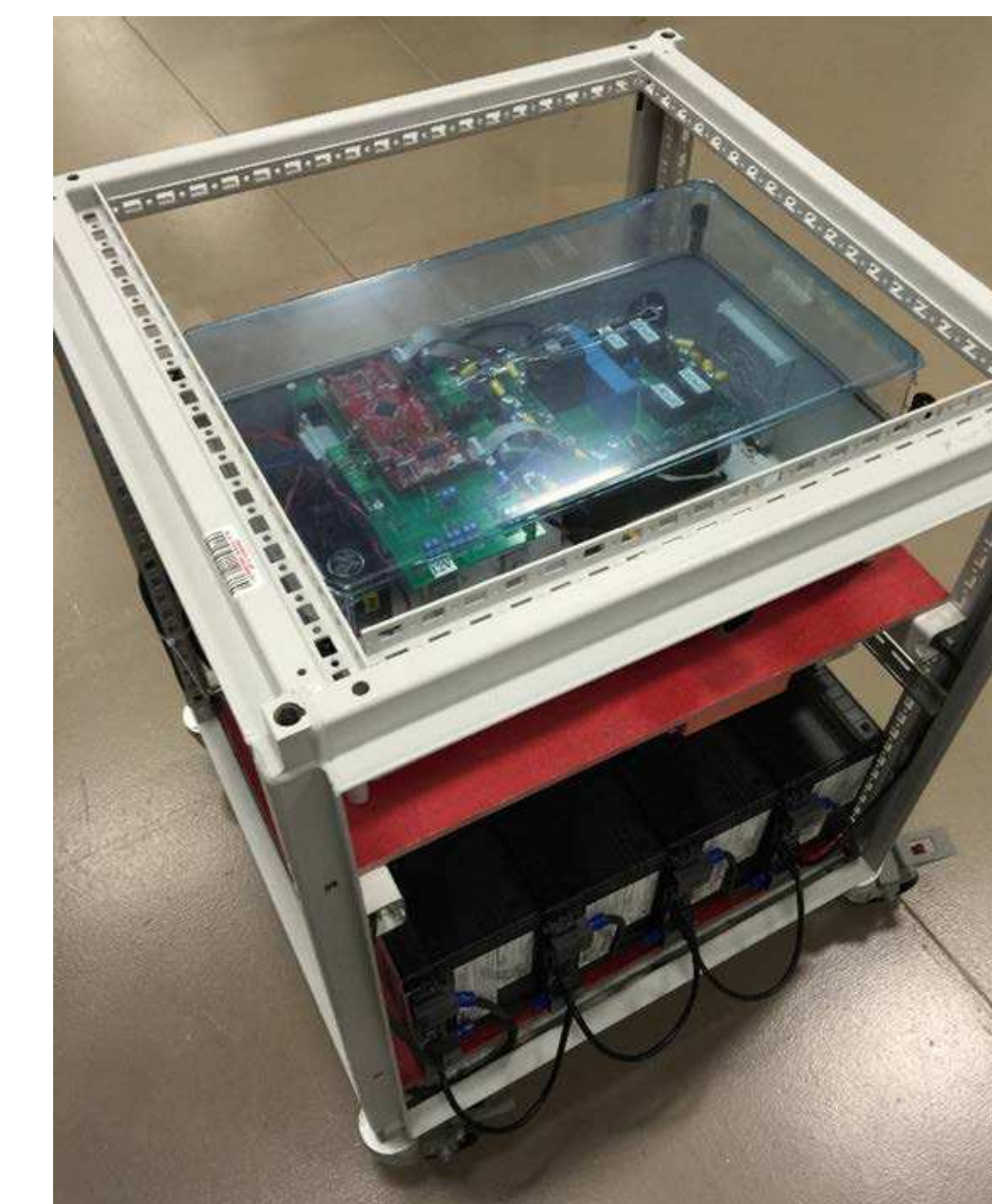
DESD System assembled into the rack
