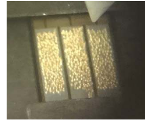
Fig. 13 SiC MOSFET with Gold Bumps on the topside for Interconnection
