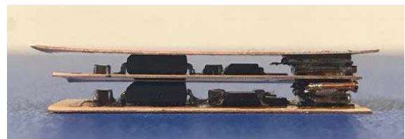
Fig. 15 Entire assembly of the whole power module with stacked structure before encapsulation
