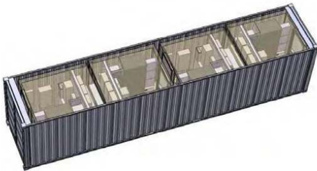
Fig. 8: The MEG was designed to fit four units in a single shipping container
