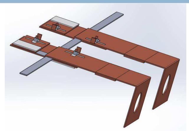
This is for showing the concept. The real design my have a U shape cooling pipe for each of the half bridge unit.
