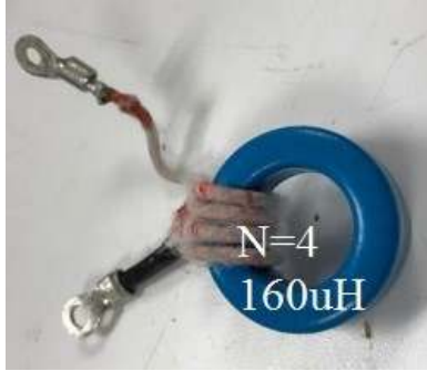
Fig. 6. EPCOS T38 saturable inductor core with N=4 turns.
