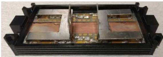
Fig. 4 An  $8.5kV/200A$  diode module (*D1-8500-200*) used high-side device in DPT
