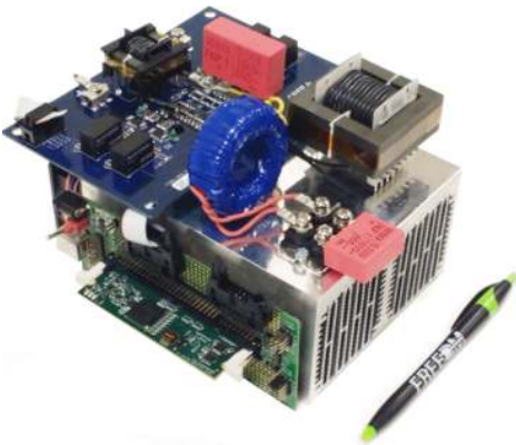
Fig. 5: Partial power rated charger realized in laboratory - Scaled down prototype.
