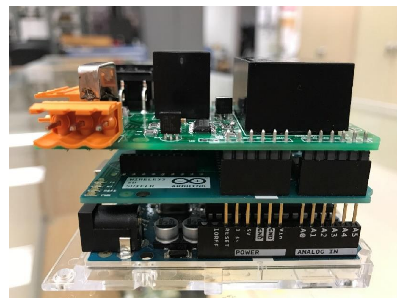
Fig. 4 Load Agent Setup for HEMS System Testbed
