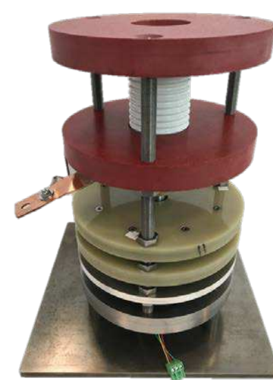
Fig. 4: Ultra-fast mechanical switch
