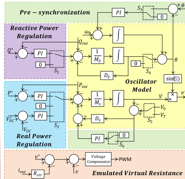
Control structure of a Low voltage oscillator module (LVOM)
