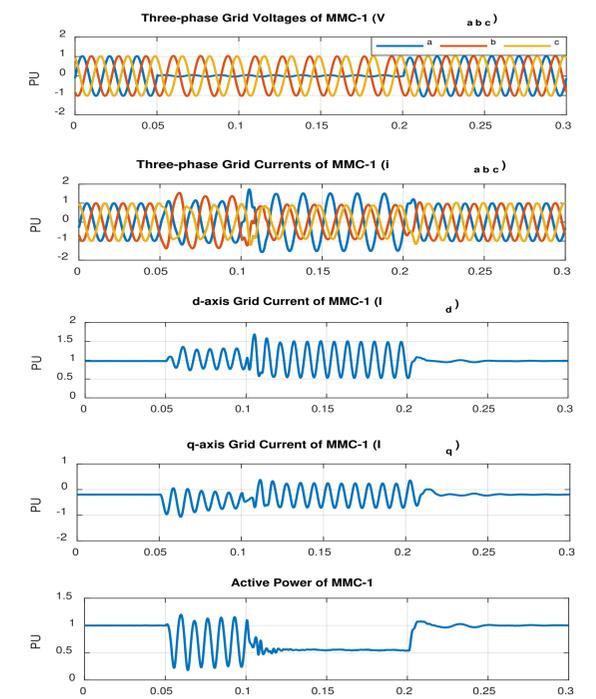
Fig. 5. RTDS results of the MMC-1 under unbalanced grid conditions
