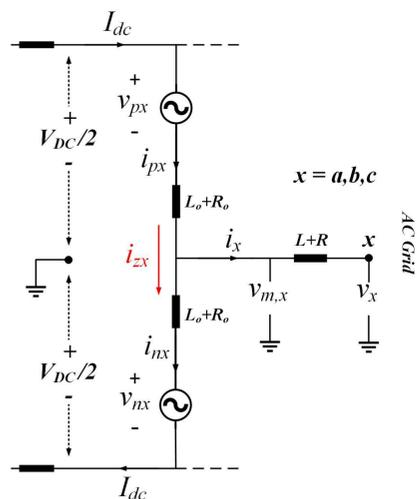
Fig. 2. Single-phase equivalent circuit of the MMC
