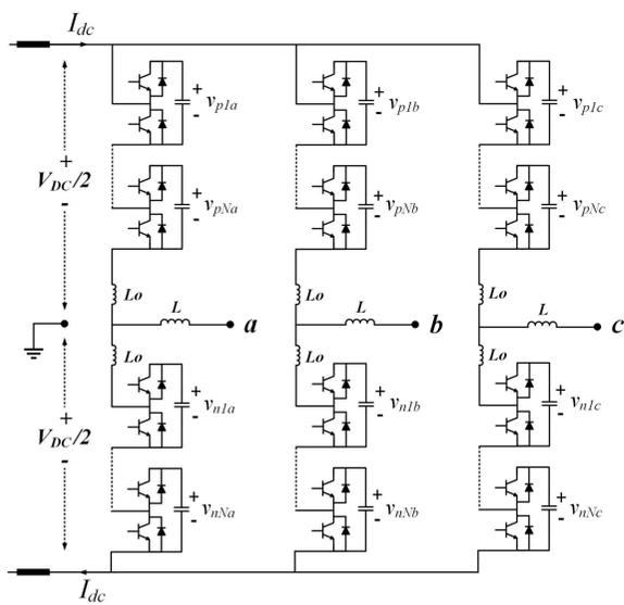
Fig. 1. Three-phase Modular Multilevel Converter (MMC) configuration
