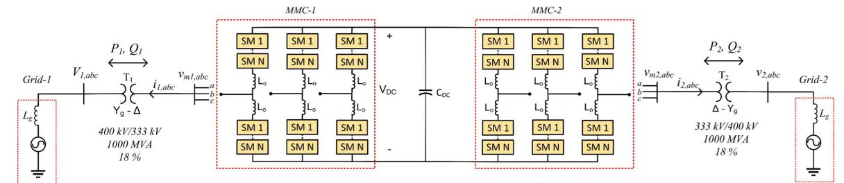
Fig. 4. Back-to-Back MMC system based HVDC
