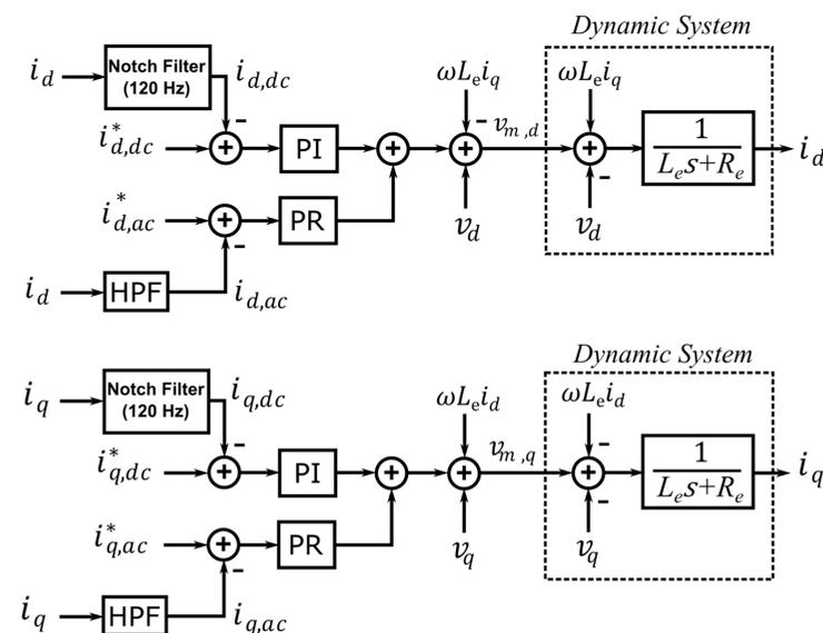
Fig. 3. ICC under balanced and unbalanced grid conditions
