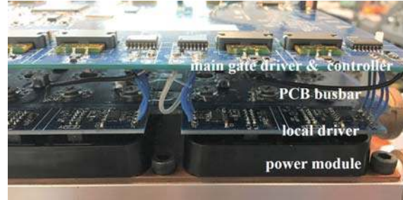
Fig. 12: Position of the 'local driver' and 'main driver' to build the split gate driver.
