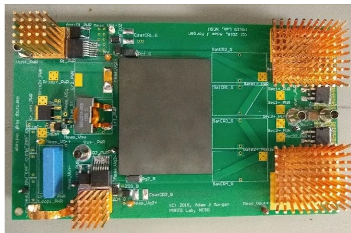
Fig. 1: Self-Oscillating LLC Resonant Converter in Voltage-Drive Configuration
