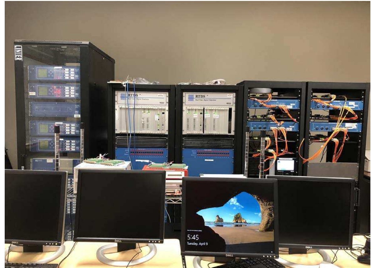
RTDS set-up with multi-vendor PMU racks
