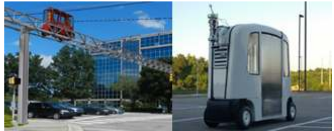
Fig. 1. EcoPRT conceptual implementation (left) and prototype (right).
