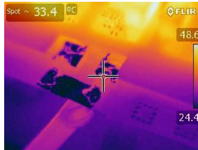
Temperature of TVS under different leakage current
