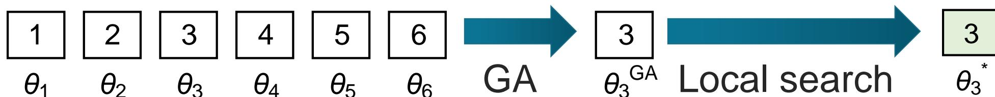
Step 1. Select 6 parent sets of  $\theta$  values for GA algorithm based on the fitness  $\Gamma$ .
