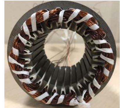
Figure 1: (Left) FEA Model of Phase A of Asymmetric Bar Winding. (Right) SSWD Winding Prototype.
