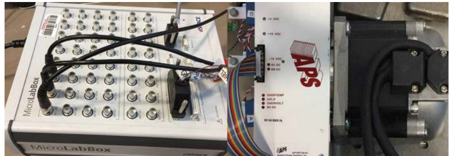
Figure 1: Dspace control, inverter, and SPM motor under test.
