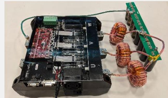
Non-isolated interleaved buck prototype
