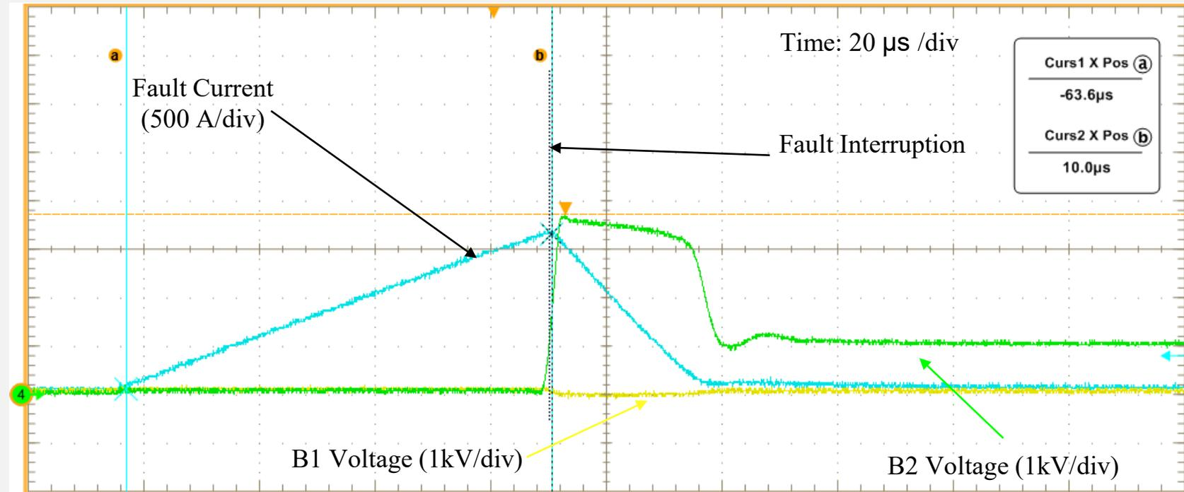
$V_{DC} = 1000\text{V}; L_{sys} = \sim 40\mu\text{H}$
