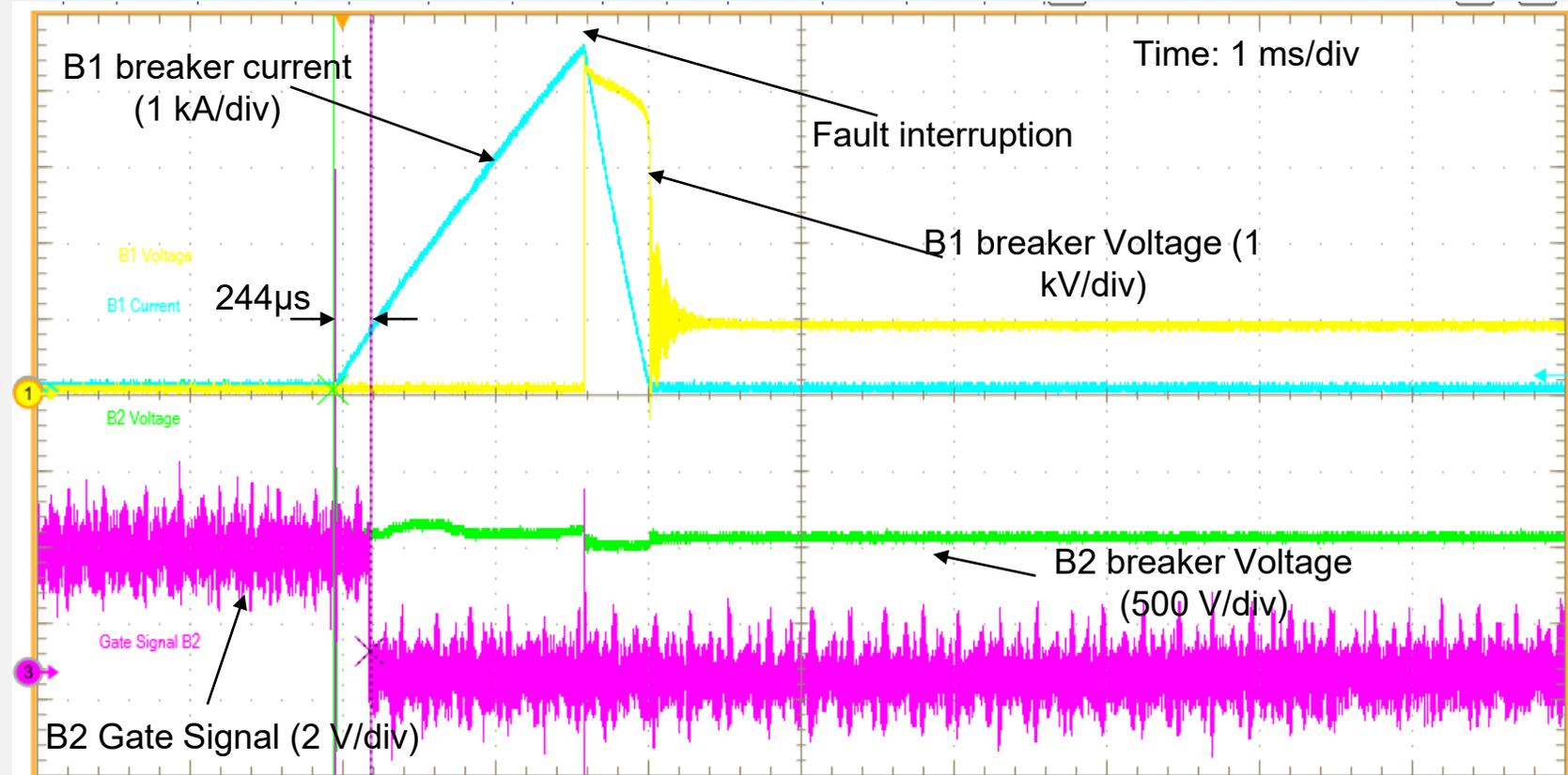
Successfully validated tripping/ turn-off of both breakers and fault isolation for a fault within switchgear cabinet
