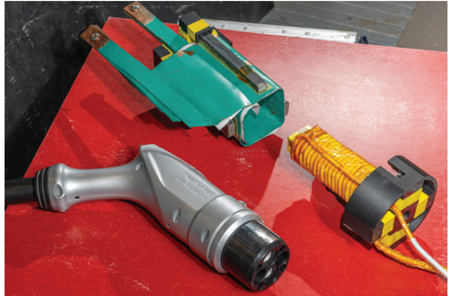
Magnetic plug next to conventional, conductive EV interconnect.
