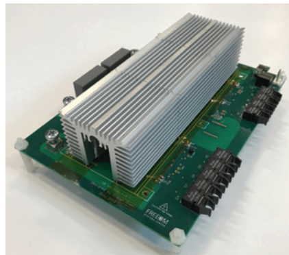
10kVA AC-DC converter prototype.
