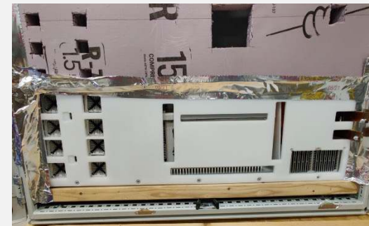
Module thermal test with cabinet cooling, and CFD simulation to identify equivalent flow resistance
