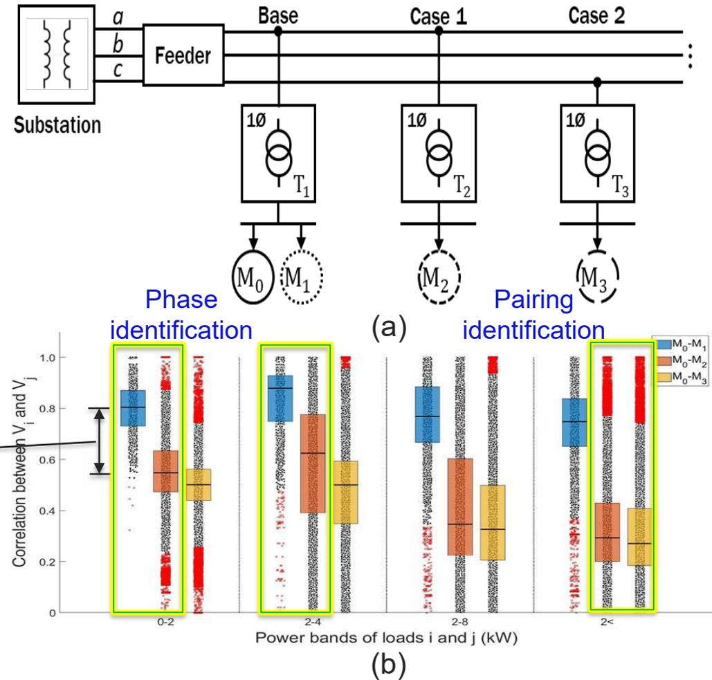
[Fig. (a) An illustration of meter locations, (b) Boxplots of PCCs between  $V_i$  and  $V_j$  for a real feeder.]
