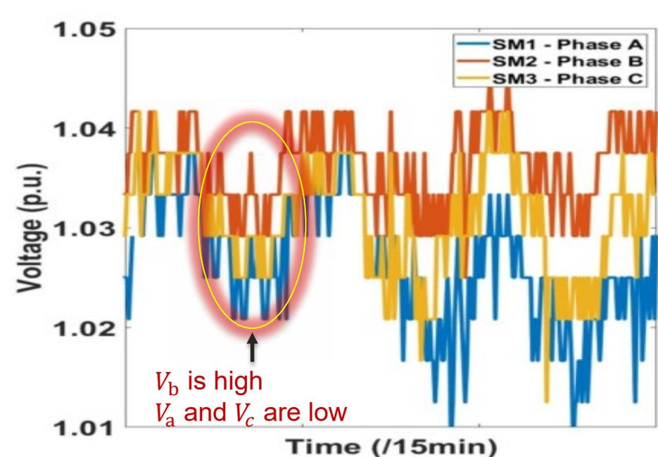
(b) Voltage profiles for meters on **different** phases
