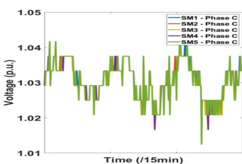
(a) Voltage profiles for meters on the **same** phase
