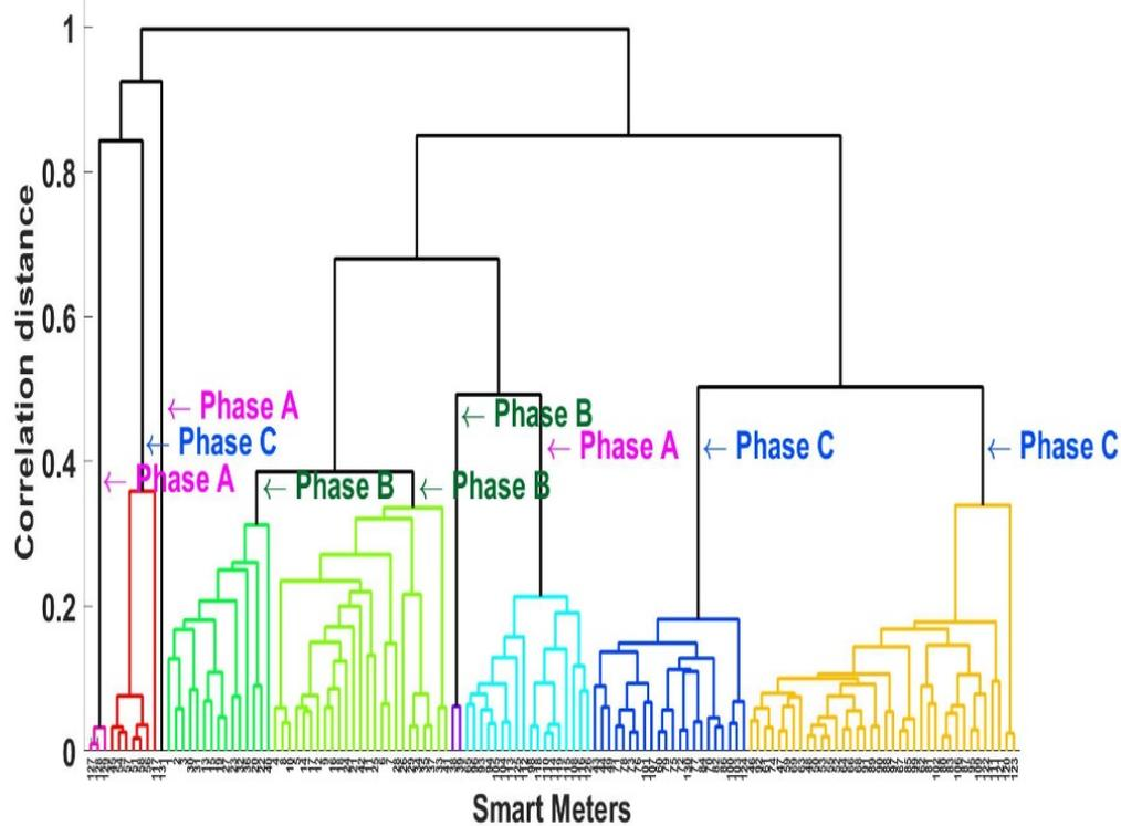
[Fig. Hierarchical clustering result of a real feeder.]
