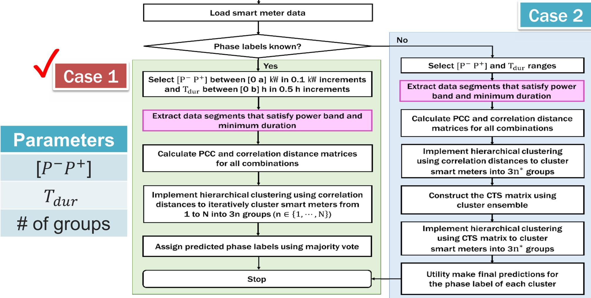
[Fig. Flowchart of the data-segmentation based phase identification methodology.]
