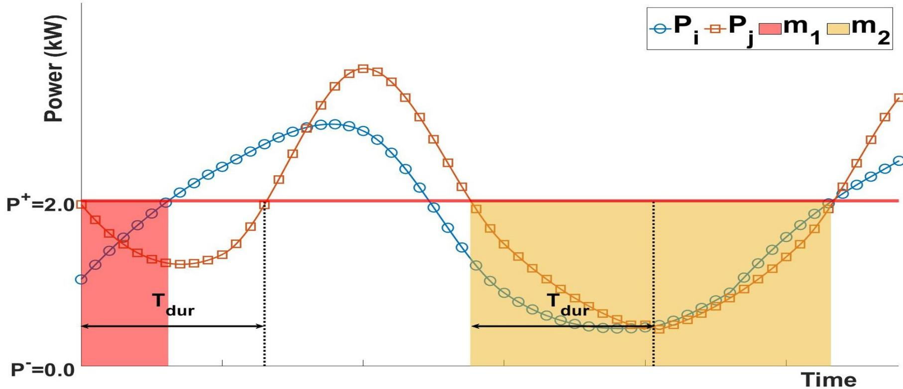
[Fig. Data segments selection between the real power of the  $i^{th}$  and  $j^{th}$  and meters.]
