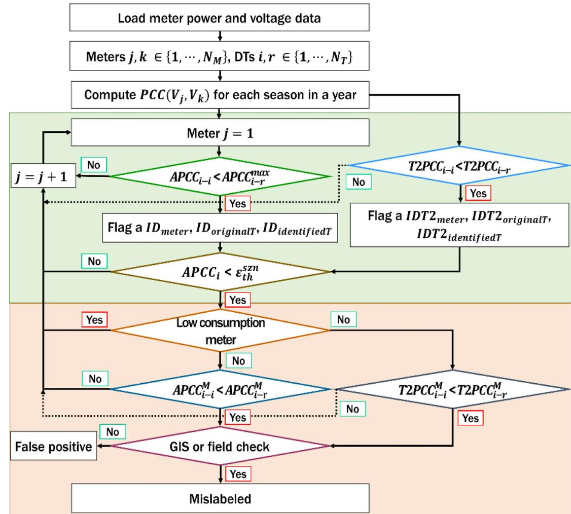
[Fig. Flowchart of the data-segmentation based, two-stage transformer-meter pairing identification algorithm.]
