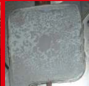
"Bake out" or "caking" Oil/filler separation "Pump out"
