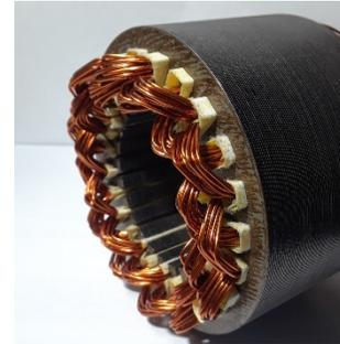
Scaled prototype of ADTP winding
