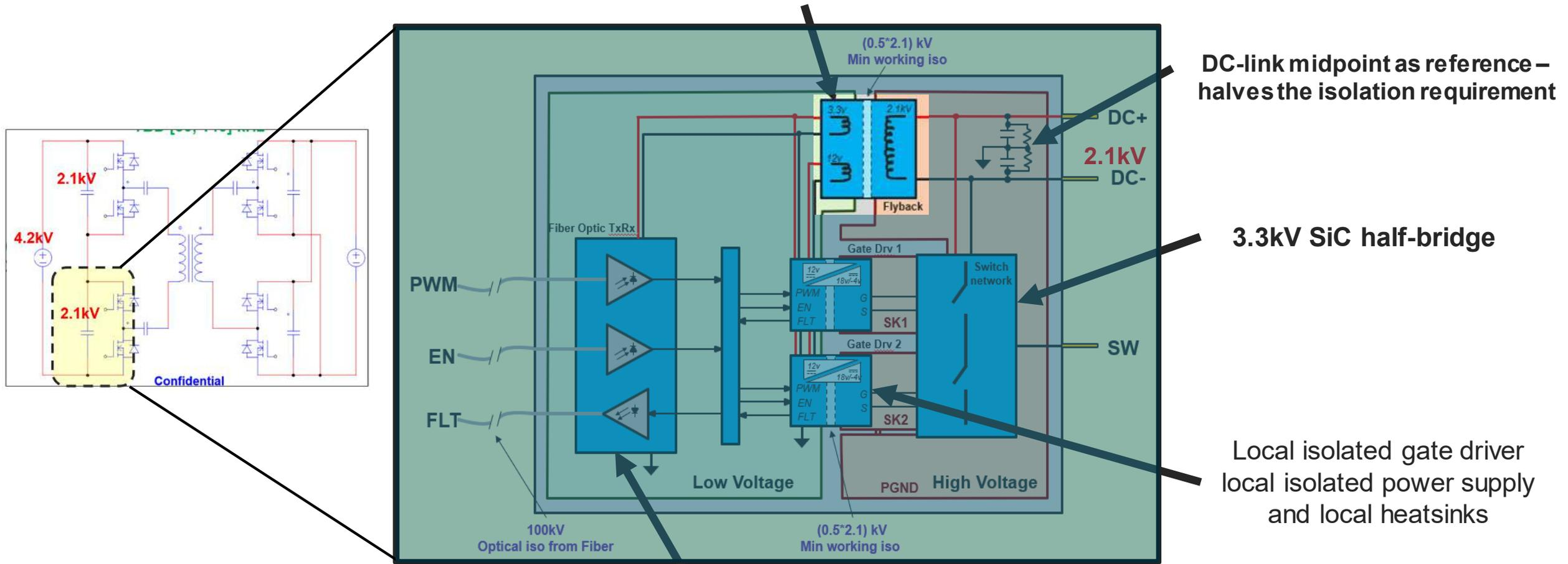
DC-link midpoint as reference – halves the isolation requirement
