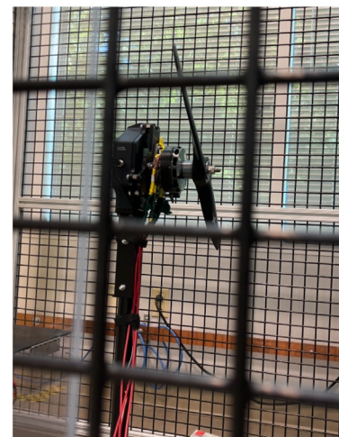
Prototype on the thrust measurement stand
